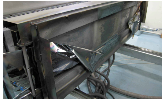
Folienriss in Sunplugged's Rolle-zu-Rolle CIGS Maschine
