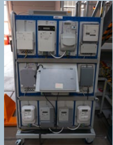
Smart Meter, AIT SmartEST Labor
