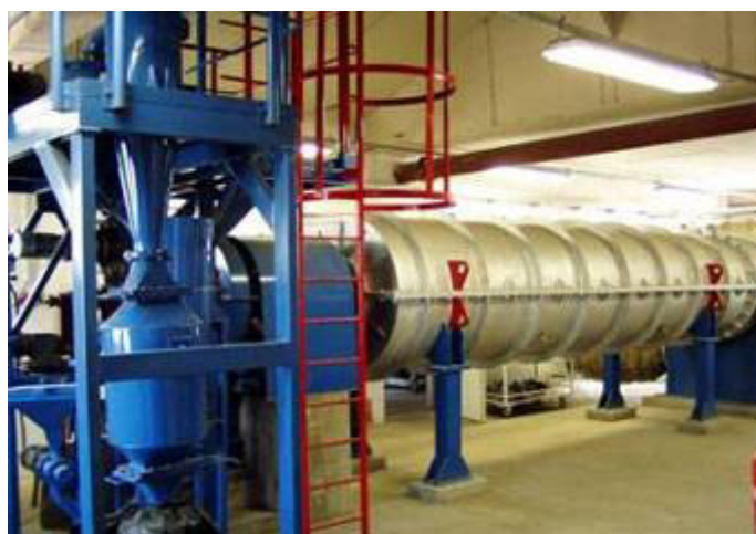
Figure 81: Rotating kiln char process of 3R Agrocarbon (Photo 3R Agrocarbon)
