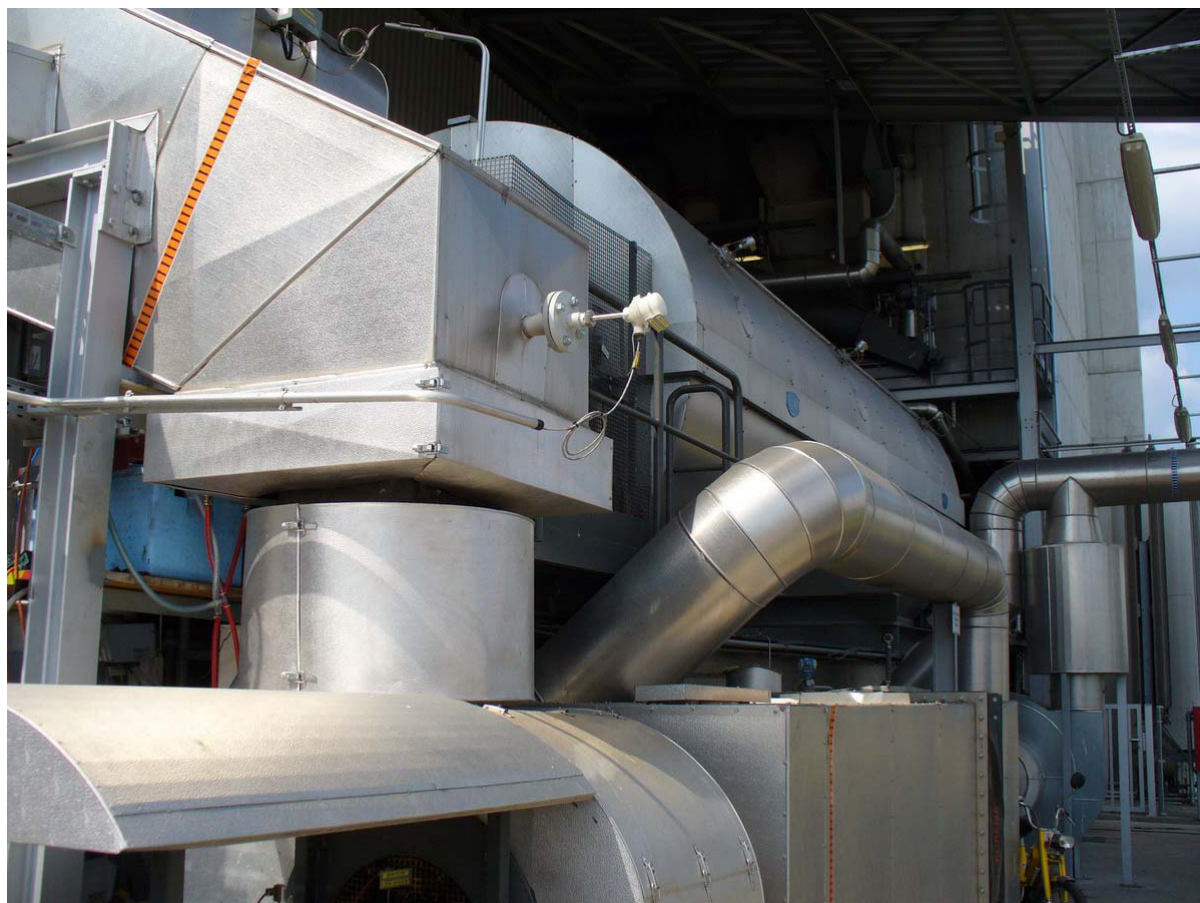
Figure 79: EVN Pyrolysis plant, detail of the rotating kiln reactor (photo: Lauer)
