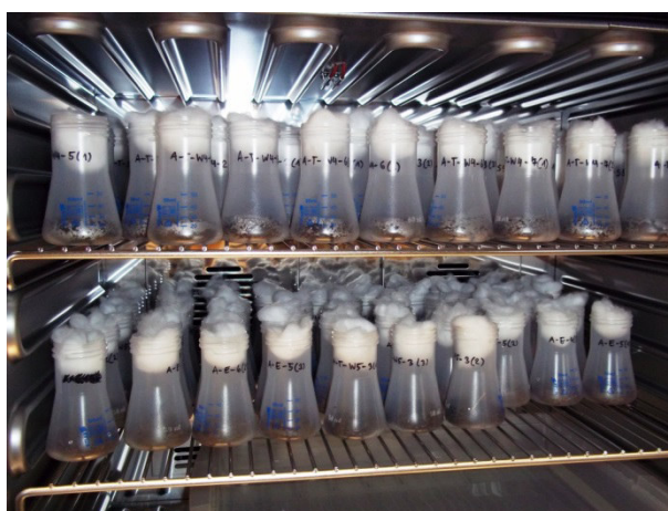
Figure 19 Erlenmeyer flasks filled with soil-BC mixtures. The flasks are placed inside the incubator. The flasks were plugged with cotton balls to prevent contamination.
