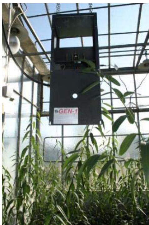
Figure 18 Methane combustion unit for ^{13}\text{C} labeling of the plants used for the incubation experiment.
