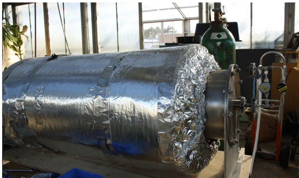
Figure 4: Pyrolysis reactor used for the biochar production of materials used later on in the microlysimeter experiment.
