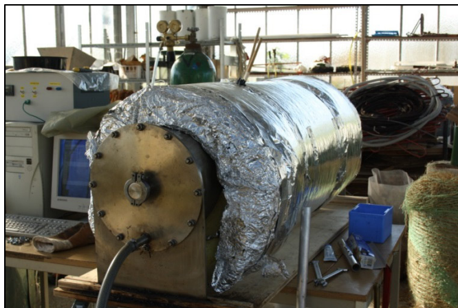
Figure 45 Stainless tube furnace unit in Seibersdorf, NÖ.
