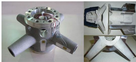
Fig. 7. Machined wheel hub equipped with strain gauge sensors and two half-cut views to prove the casting process
